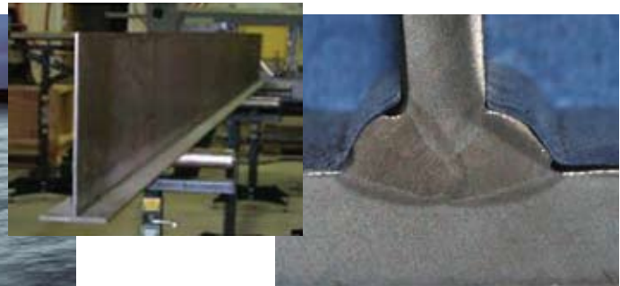
Close-up photo is an HSLA-80 web welded to an HSLA-80 flange using hybrid laser arc welding (courtesy Applied Thermal Sciences)
