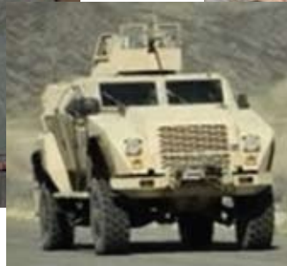
Driver side windshield is a spinel-based transparent armor
