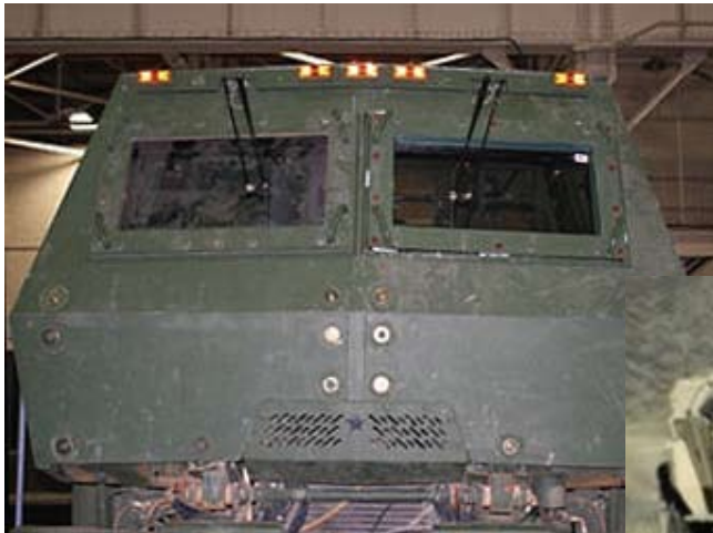
Driver side windshield is a spinel-based transparent armor
