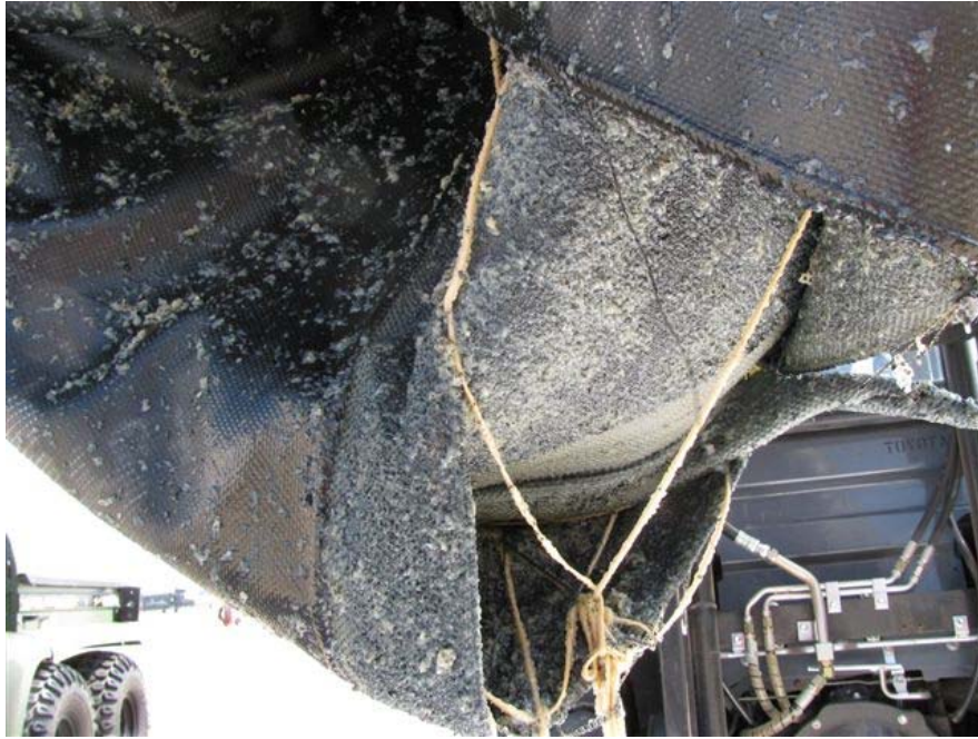
Figure 34. External View of the Degraded Fuel Bladder – View 1
