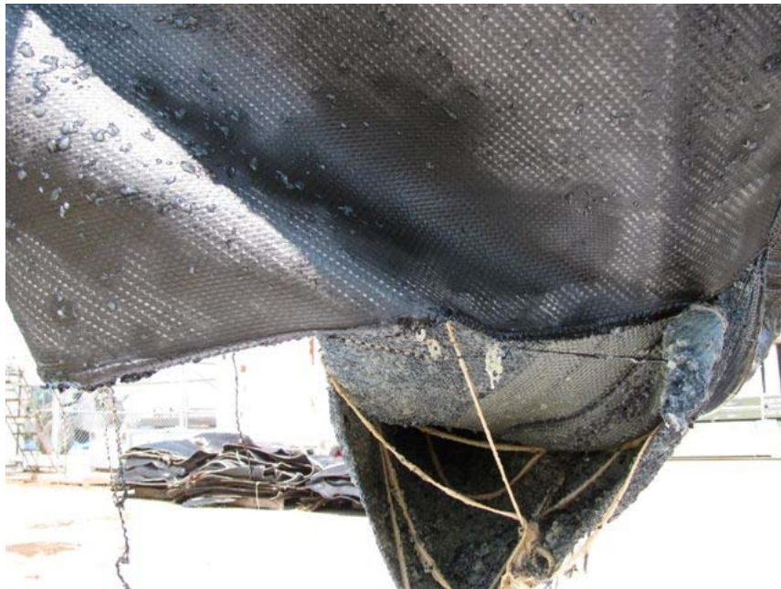
Figure 35. External View of the Degraded Fuel Bladder – View 2
