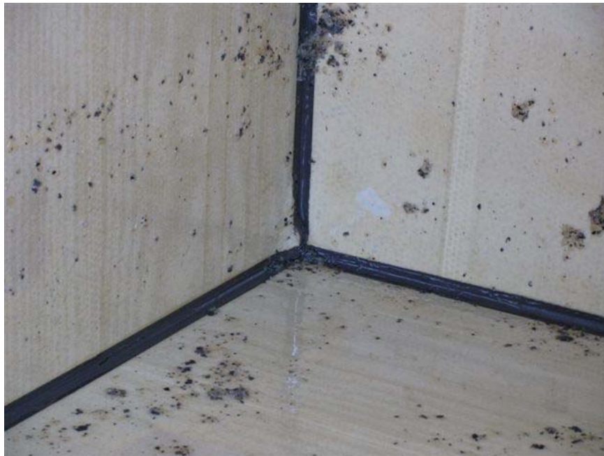
Figure 31. Unknown Contaminant in Fuel Bladder
