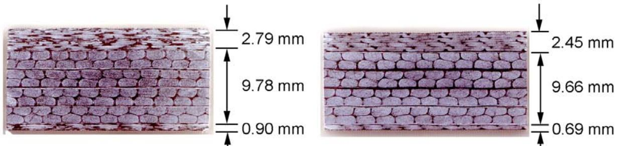
**Figure 4. Cross-sections (sectioned at 90°) of complex laminates with two ply drops, thick side, layup from top surface [(±45)<sub>4</sub>/(90/0/0/90)<sub>4</sub>/(±45)]; Fabric M ±45's (left), Fabric L ±45's (right).**
