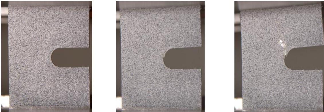
**Figure 3. Series of photographs showing the loading history of a composite specimen tested in the MSU-IPL in a rotational load path (speckled paint applied for image analysis)**
