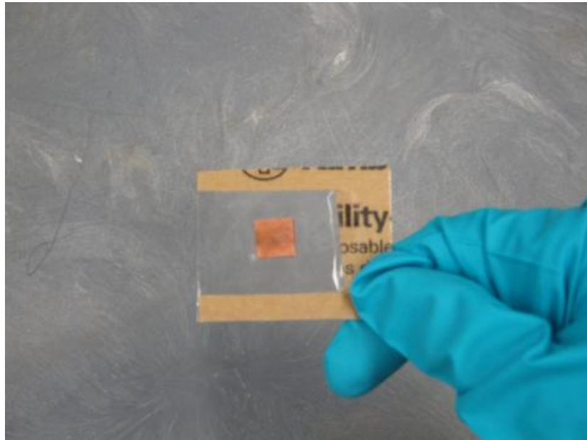
Figure 23: Radioactive single crystal copper sample
