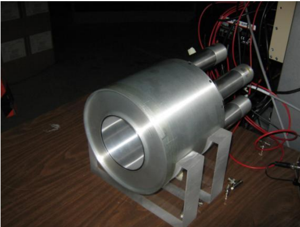
Figure 6: Picture of NaI ring detector used for 3\gamma/2\gamma experimentation.
