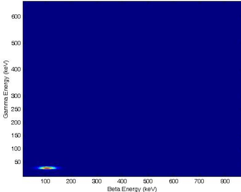
**Figure 1. Spectrum of a sample containing only  $^{131\text{m}}\text{Xe}$ —6.9-hour irradiation, 73.4-hour decay, 87.6-hour count**
