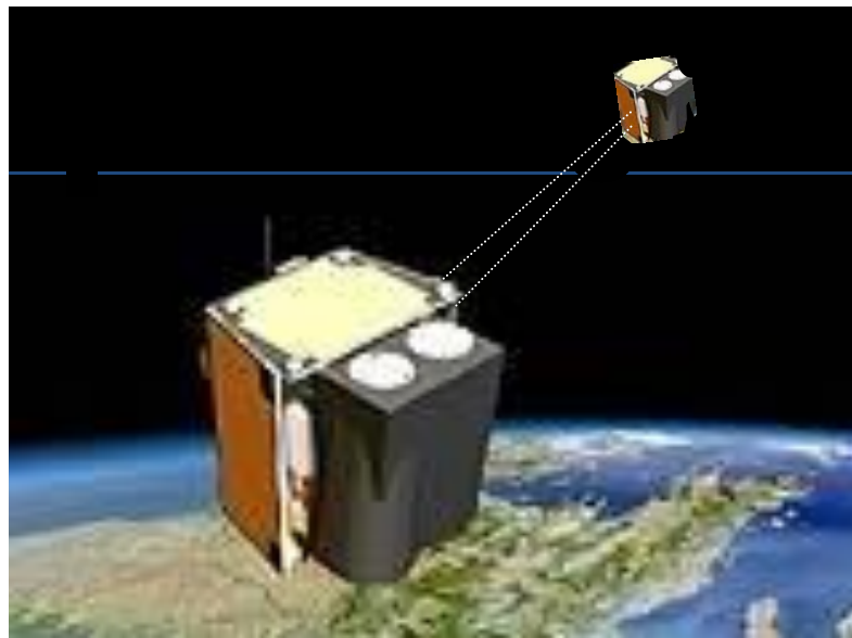
Figure 1. Droplet Stream Propulsion Concept in which Momentum is Exchanged Between Satellites Creating a Continuous Displacement Force from the Reference Orbit Centerline.
