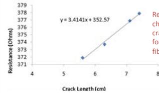
Resistance changes as crack grows for a carbon fiber sample
