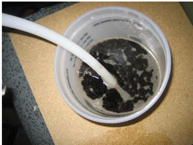
Figure 13. Resin at inlet with bubbles after mixing.
