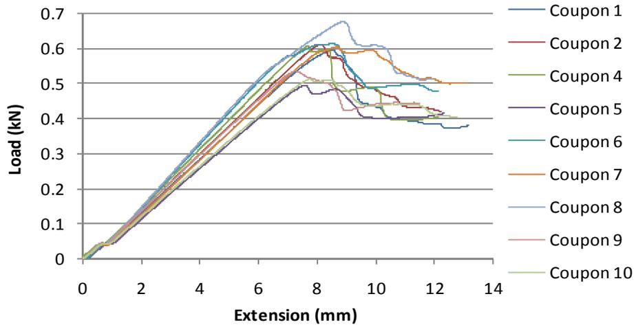
Figure 38. Load-extension data for fiberglass coupons with CNTs.
