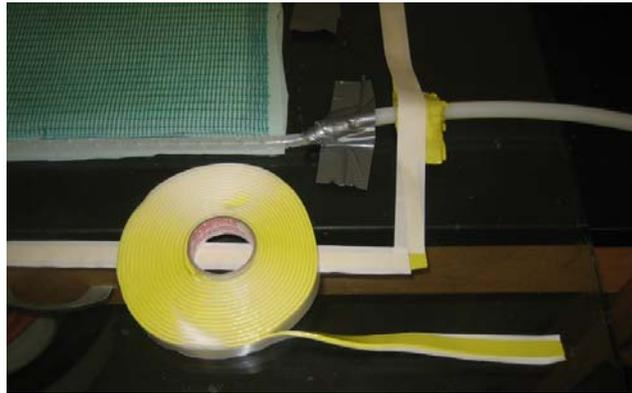
Figure 10. Vacuum tape used to seal the sample setup.
