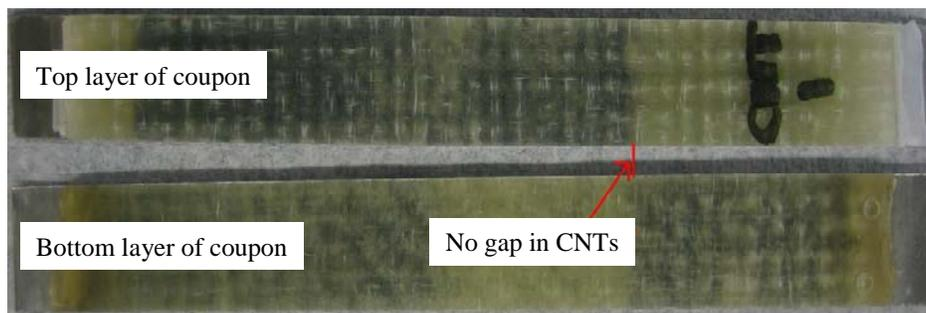
Figure 36. Fiberglass coupon with continuous layer of CNTs.
