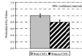
Application of CNTs along carbon fiber composite interface significantly improved Mode II fracture toughness
