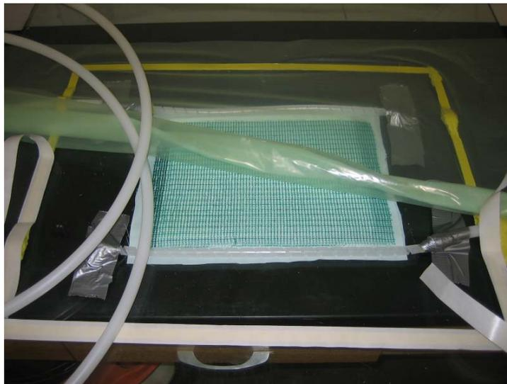
Figure 11. Rolling out the plastic sheet used to form the vacuum bag.
