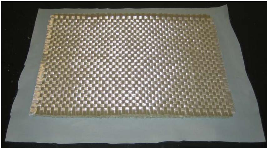
Figure 6. Bottom five layers of a sample.
