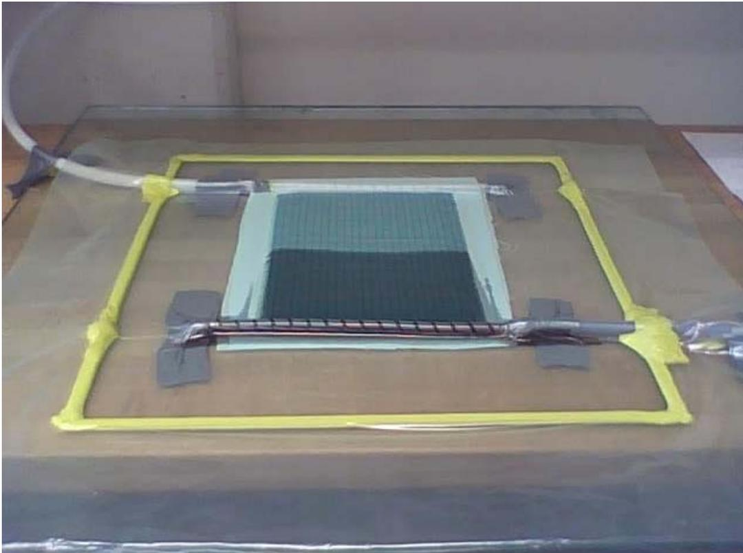
Figure 14. Resin running through a sample evenly.
