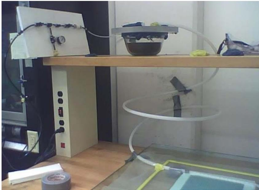
Figure 8. Gage board and resin trap.
