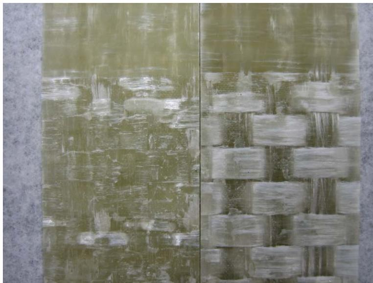
Figure 45. Surface view of crack propagation path in fiberglass coupon without CNTs.
