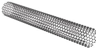
Figure 1. Single-walled carbon nanotube.<sup>9</sup>
