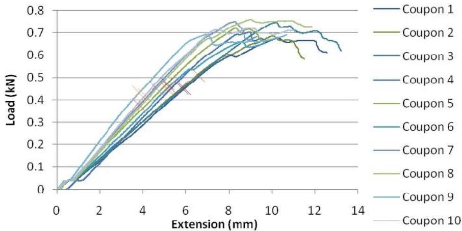
Figure 39. Load-extension data for fiberglass coupons without CNTs.
