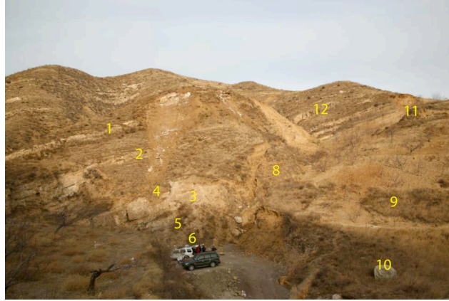
Figure 10. A photograph of the Dec122007 test site after the explosion from BIT Blast’s news bulletin. Minor landslides are seen on the side of the hill. Numbers in the figure mark some of the surface features that are recognized in the Google Earth™ image (Figure 11).
