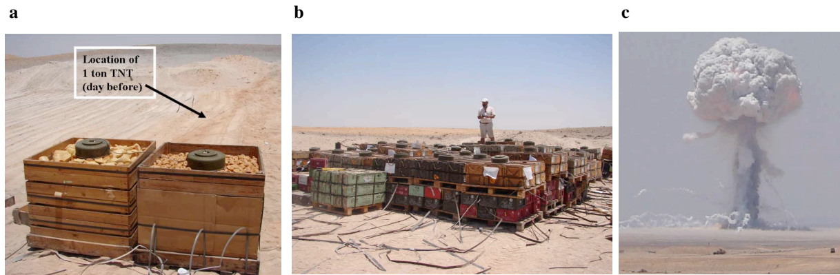
Figure 13. Design of the experimental explosion #8 of 1 ton of Composition B (a), detonated ~10 minutes after the largest shot, explosion #7, in the series, in which outdated ammunition was destroyed by mines of 8.63 tons of Composition B (close to ~10 ton TNT equivalent) (b); as observed from a safe position at Post 604, at 5.3 km (c).
