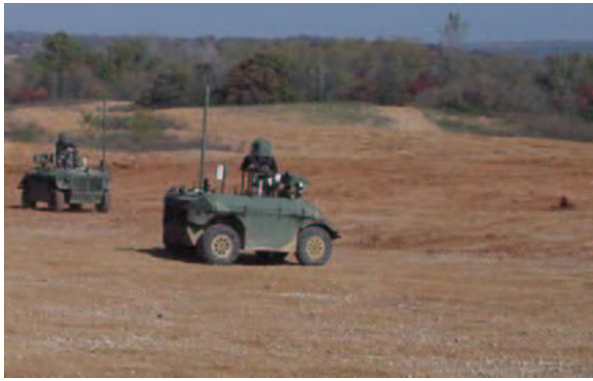
Fig. 1. Two Demo III vehicles performing an autonomous mission
