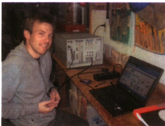
Figure F2. The Hewlett-Packard E1437A 20 Msamples/s, analogue-to-digital converter, and laptop computer used sample the electromagnetic emissions.
