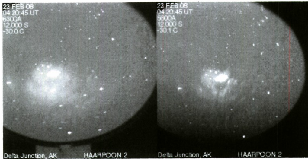
Figure O1. 630.0 (left) and 557.7 (right) nm wide-field images of HAARP-induced optical emissions from the \sim 90^\circ FOV HAARPOON system at Delta Junction during the experiment on 23 Feb 2008. Note that north is toward the bottom of these quick-look images.
