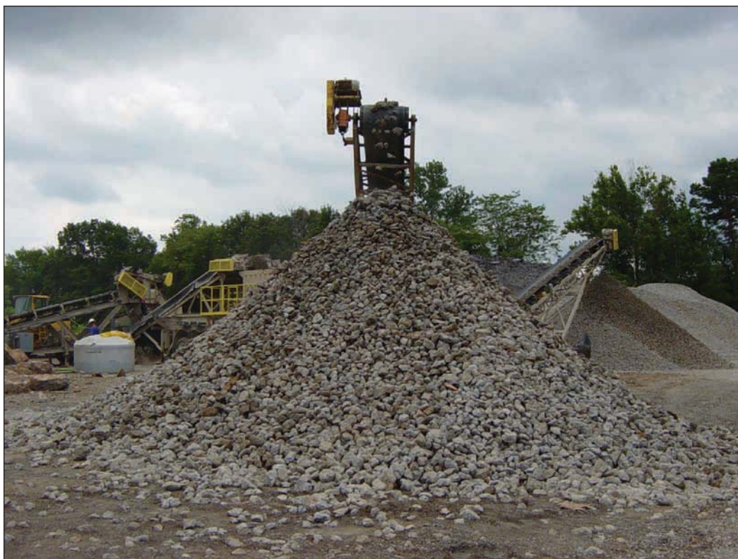
Figure 3.6 Fort Campbell's Concrete Grinding Creates Reusable Gravel
