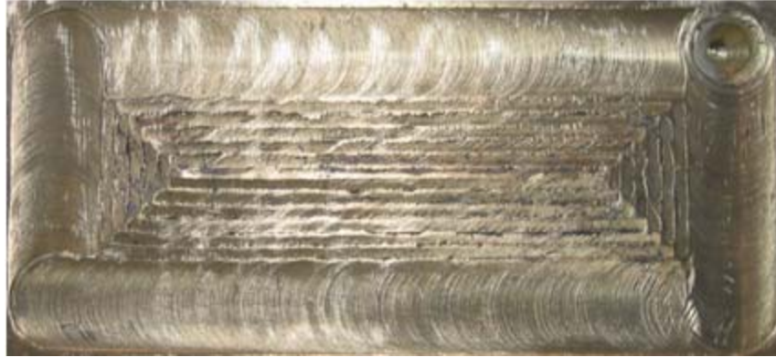
Figure 6. Example of a rectangular spiral pattern used for FSP of multiple pass plates.
