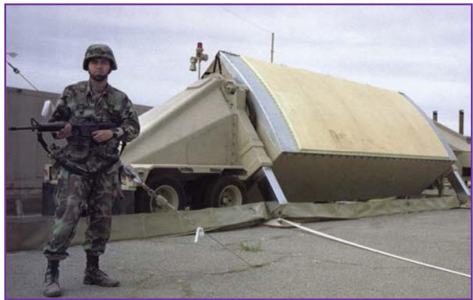
AN/TPY-2 RADAR. This transportable X-band radar is currently deployed to Japan to aid in detecting and tracking potential threats in the Pacific region.
