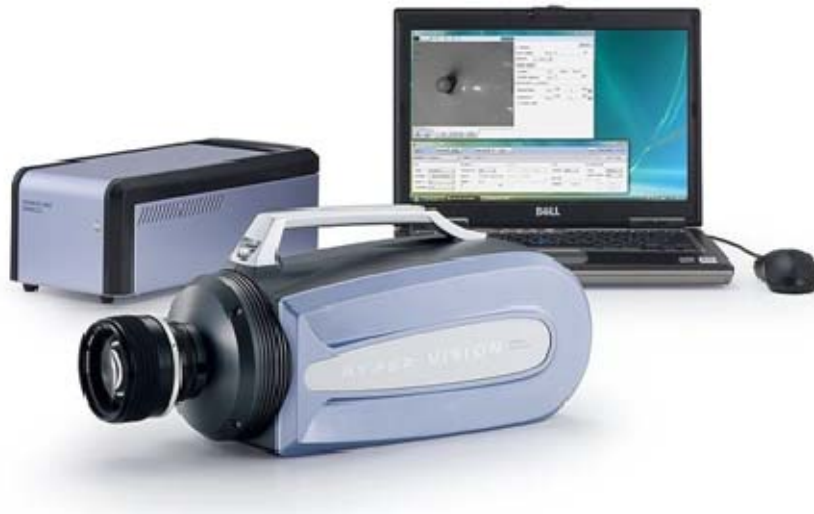
Figure 18. Shimadzu Hyper-vision 2 Camera with Power Supply and Software
