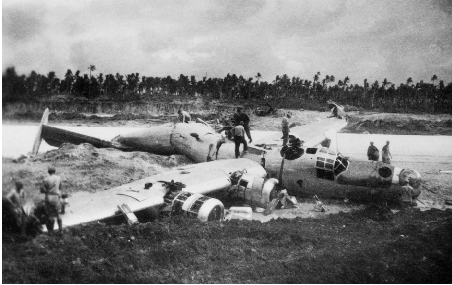
Figure 3. Once its structural integrity was lost as it left the coral airstrip, this 5 th Bomb Group B-24 displayed the catastrophe that attended runway mishaps (A.B. Goldberg collection)
