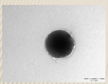
Encapsulated particles via Supercritical Technology Nanoscale particle: 150nm With 5-10 nm thickness
