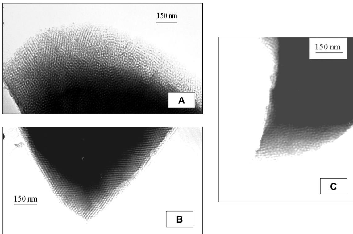
**Figure 2.** TEM images of ferritin-containing samples at the specified ferritin concentrations: A) 1 wt% ferritin loading; B) 5 wt% ferritin loading; C) 10 wt% ferritin loading. Reaction conditions: TEOS infusion at 40°C, 126 bar; calcination for 6 hours at 400°C
