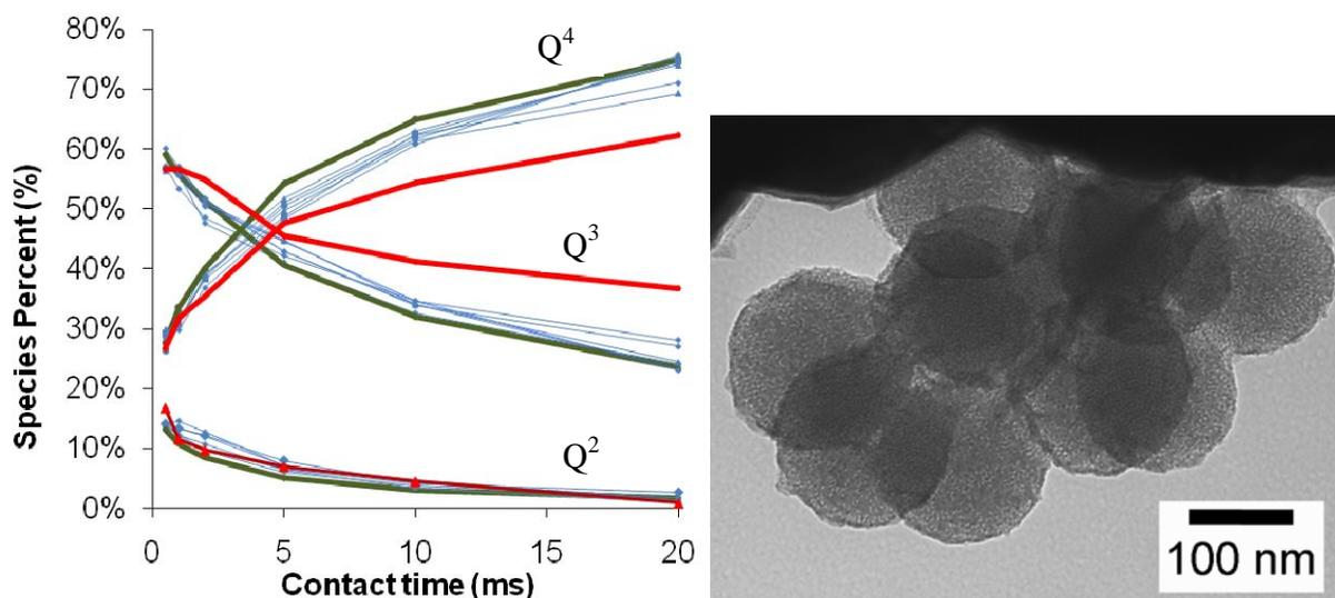
**Figure 7:** Left: Deconvoluted CP NMR for uncalcined cys-spheres (blue lines) and Grun spheres (bold red lines), Right: TEM image of mesoporous cys-spheres. Green lines indicate cys-sphere sample with highest amount of TEOS loading.
