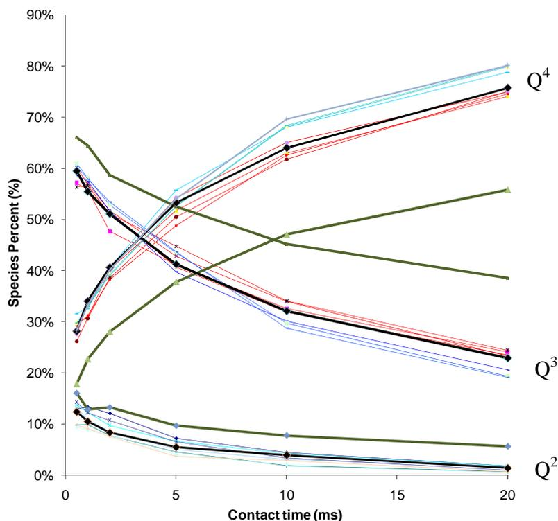
**Figure 10:** CP NMR data summarizing catalyst effect on degree of surface condensation. Light blue lines and the dark blue lines represent uncalcined silica spheres synthesized using the mixed catalyst system at pH = 7. Red lines represent spheres synthesized using cysteamine. Green lines represent silica formed without cysteamine or glutathione.
