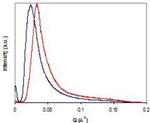
**Figure 6:** SAXS data for biodegradable block copolymer and silica composites, DL60 (blue line) indicates 64% PEO, PLA-PEO-PLA and has a d-spacing of 25 nm, DL86 (red line) represents 86% PEO, PLA-PEO-PLA and has a d-spacing of 18 nm.
