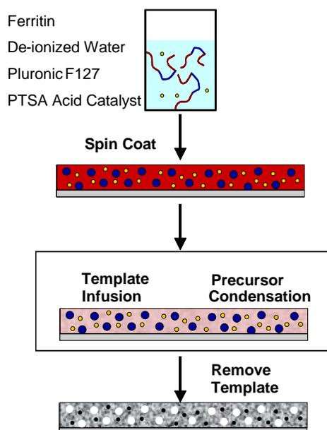
**Figure 1:** Schematic detailing the formation of ferromagnetic mesoporous silica thin films. The red continuous domain represents PEO, which is doped with ferritin (yellow spheres). The blue PPO domains are removed during calcination as is the apoferritin shell, leaving magnetic iron oxide particles (black) embedded in the mesoporous silica film.
