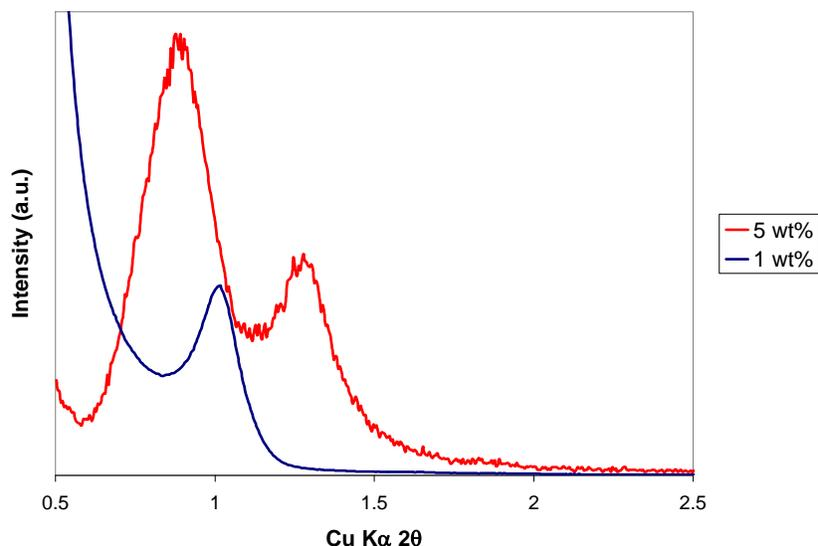
**Figure 3:** Small angle XRD of 1 wt% and 5 wt% ferritin-containing silica films
