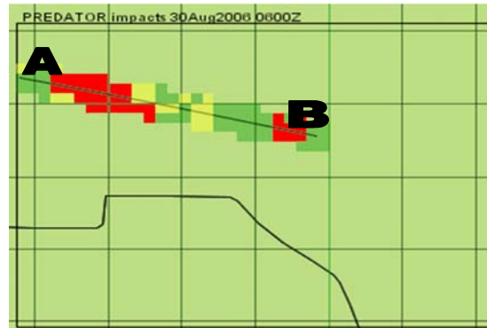
Figure 1. En-route flight weather impacts for a modeled Predator unmanned aircraft flight from A to B across southern New Mexico, 0600 UTC, 30 August 2006. Green = favorable weather conditions, Yellow = marginal conditions, and Red = unfavorable conditions.
