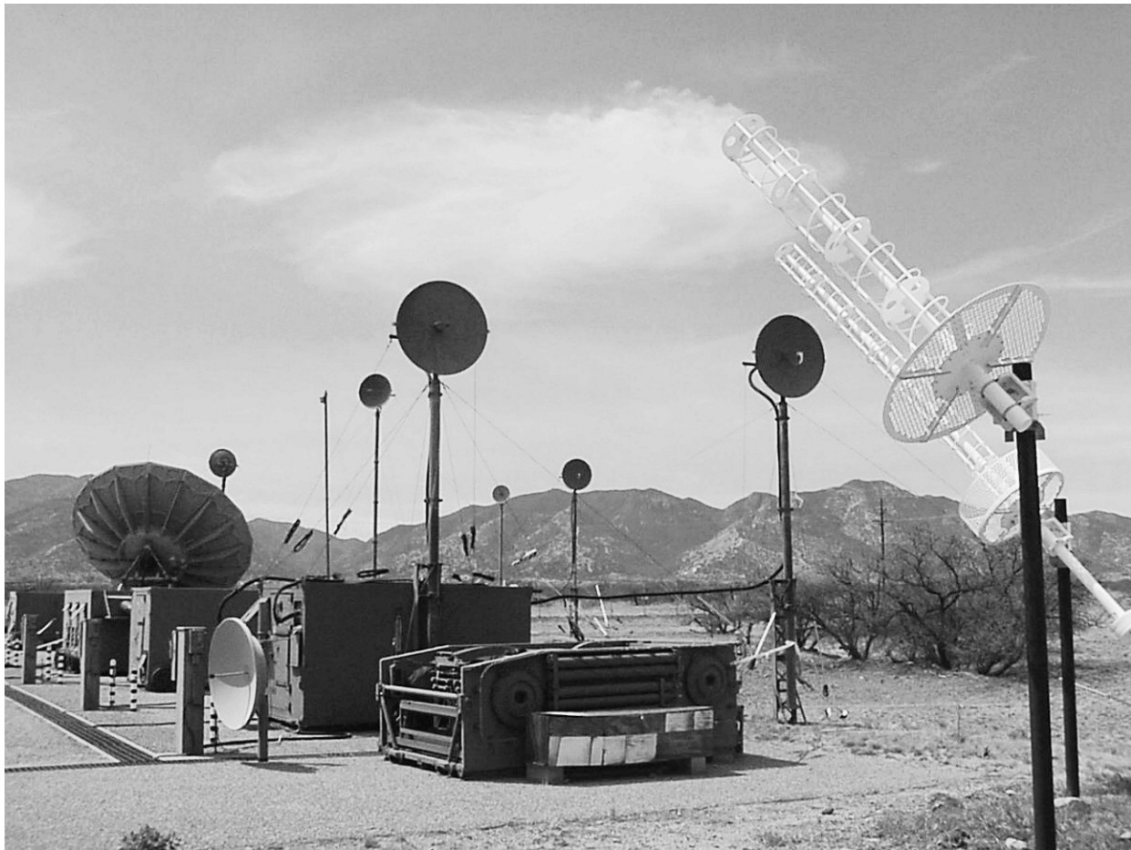
Figure 5. Operational realism Q.E.D.: The 9,500-foot-high Huachuca Mountains serve as a backdrop for a variety of Joint Interoperability Test Command test shelters and antennas, including: high-gain spiral satellite communication ultra-high frequency (SATCOM UHF) antennas; line-of-sight Army-Navy transportable radio communications-170 antennas; and, a 20-foot parabolic Army-Navy transportable SATCOM-85B antenna
