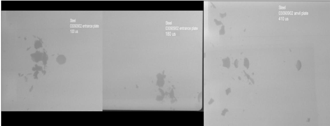
Figure 4. Steel projectile fragment progression; anvil is to the right.
