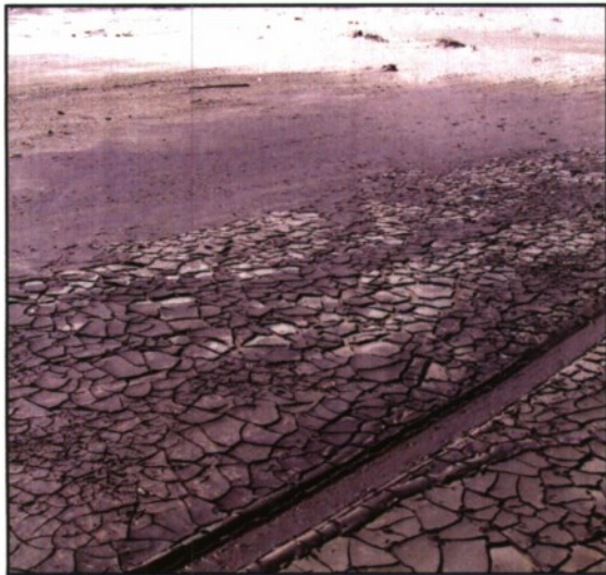
Figure 1. Tidal flat composed of sand (background) and mud (foreground). Support of the vehicle that left the track was possible because the mud is underlain by sand (as seen in background). Our research suggests that the thermal signature of sediments may be related to their geotechnical properties, potentially enabling remote characterization of trafficability on tidal flats such as this one.
