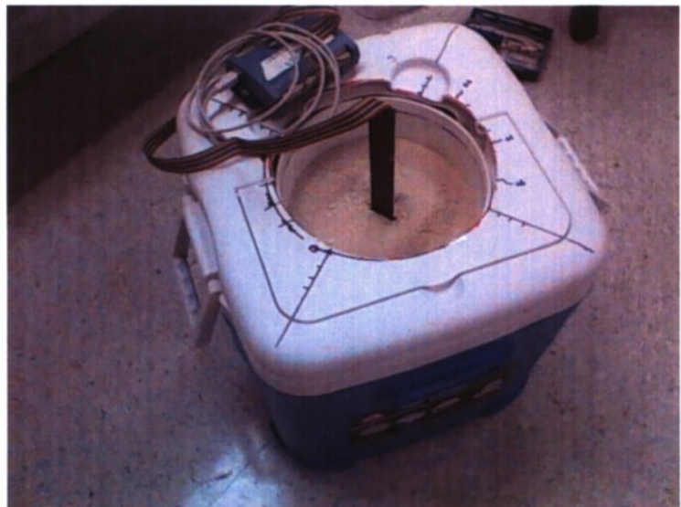
Figure 2. Bucket of kaolin clay that is insulated from horizontal heat flux by the cooler. A thermistor array is inserted into the clay in the center of the bucket. The rainbow ribbon cable transmits temperature readings to the data recorder every 5 seconds during a cooling or warming cycle. This set-up minimizes two-dimensional heat conduction.
