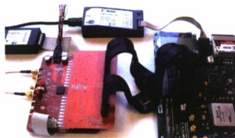
Figure 3.14: Interface setup connecting ML550 and Fujitsu DAC DK
