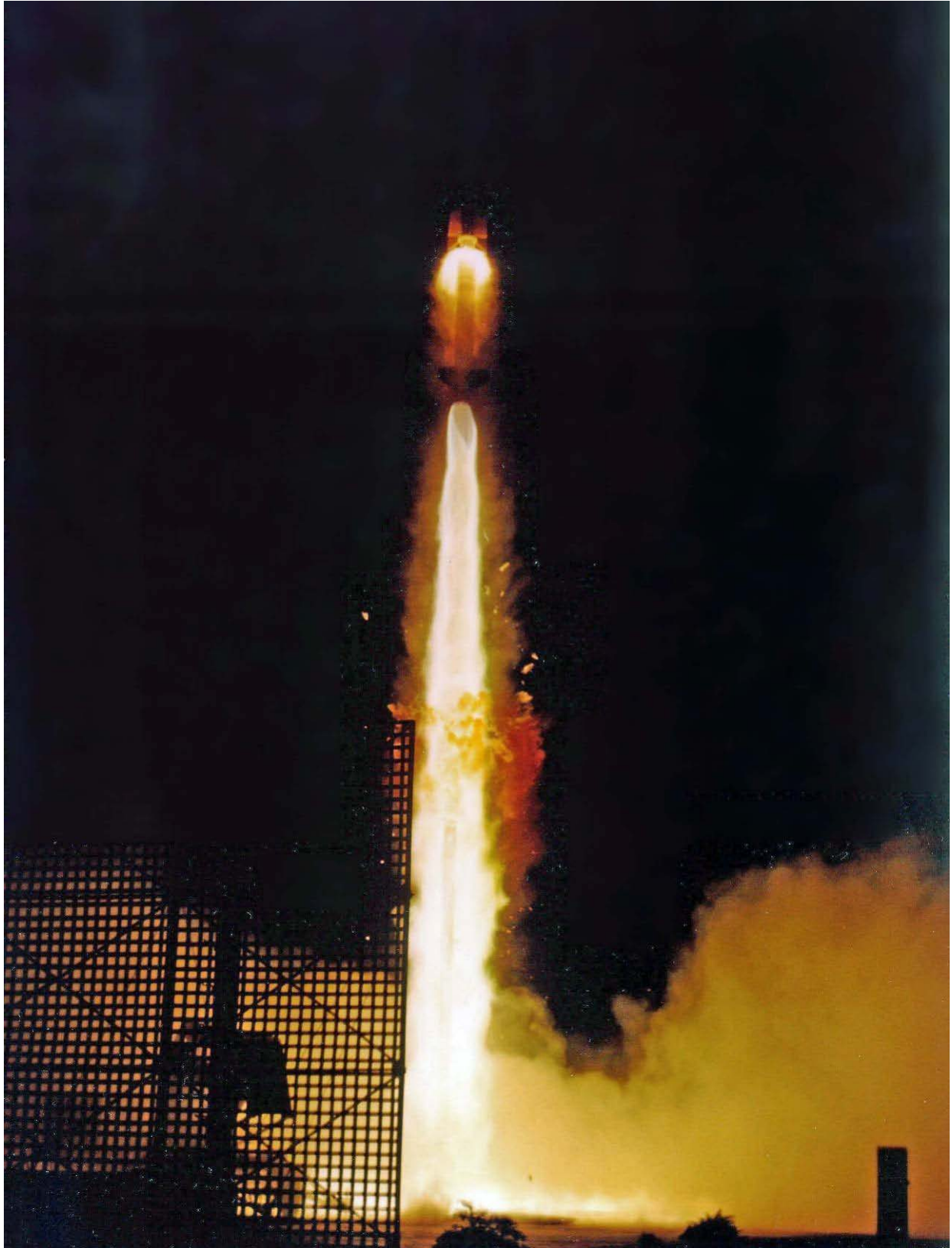
Figure 24. Launch of the HI STAR South at Woomera, Australia. The white debris is from the Styrofoam support for the booster on the rail extension.
