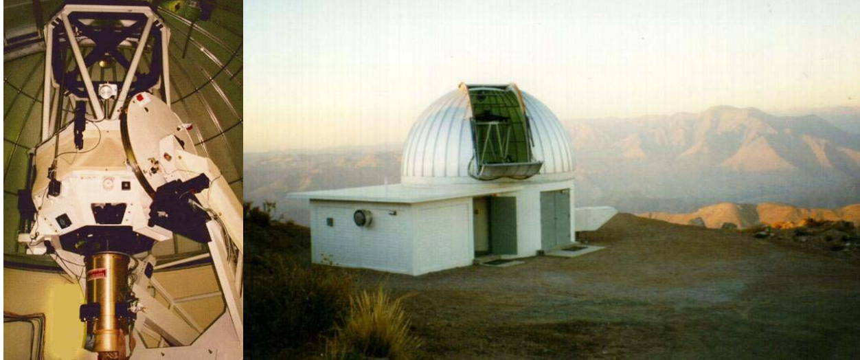
Figure 102. The 2MASS facilities. At left is the northern telescope at Mt. Hopkins in Arizona. The cylinder at the back of the telescope is the three-color near-infrared camera. The 2MASS site at the Cerro Tololo Inter-American Observatory is shown at right. These and the other images in this section are courtesy of the Two Micron All Sky Survey (2MASS), a joint project of the University of Massachusetts and the Infrared Processing and Analysis Center/California Institute of Technology, funded by the National Aeronautics and Space Administration and the National Science Foundation.
