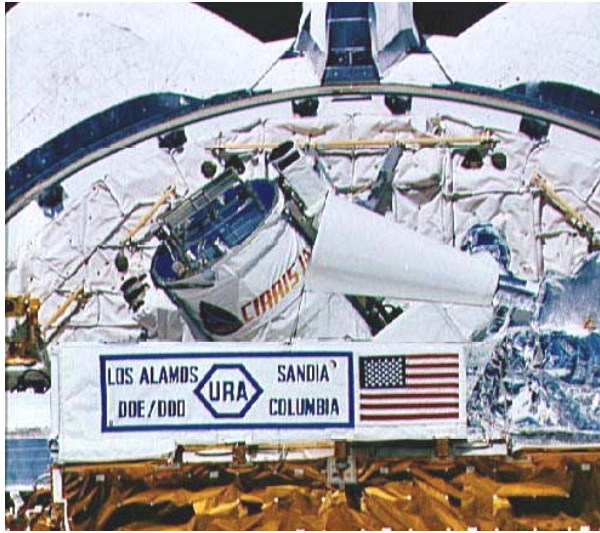
Figure 70. CIRRIS 1A in Discovery Shuttle Bay. The University of Arizona ultraviolet experiment is the horn in the foreground atop the labels. The UV, the IBSS infrared sensor and a visible sensor were on the SPAS II Pallet, a free flying platform during the mission.
