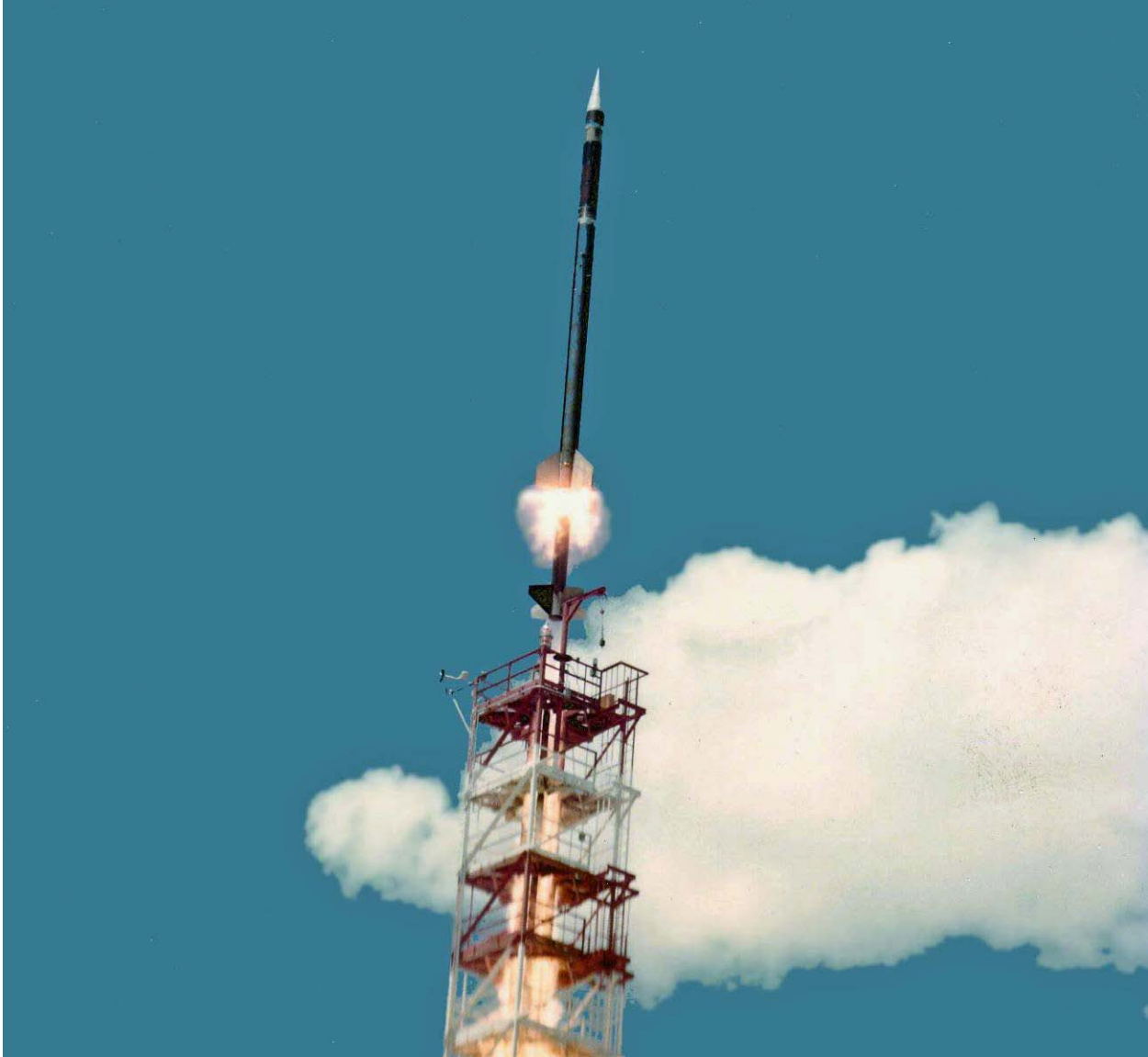
Figure 19. A daytime Aerobee 170 launch. The Nike booster and the Aerobee sustainer are ignited at the same time and separate plumes for the two may be seen.
