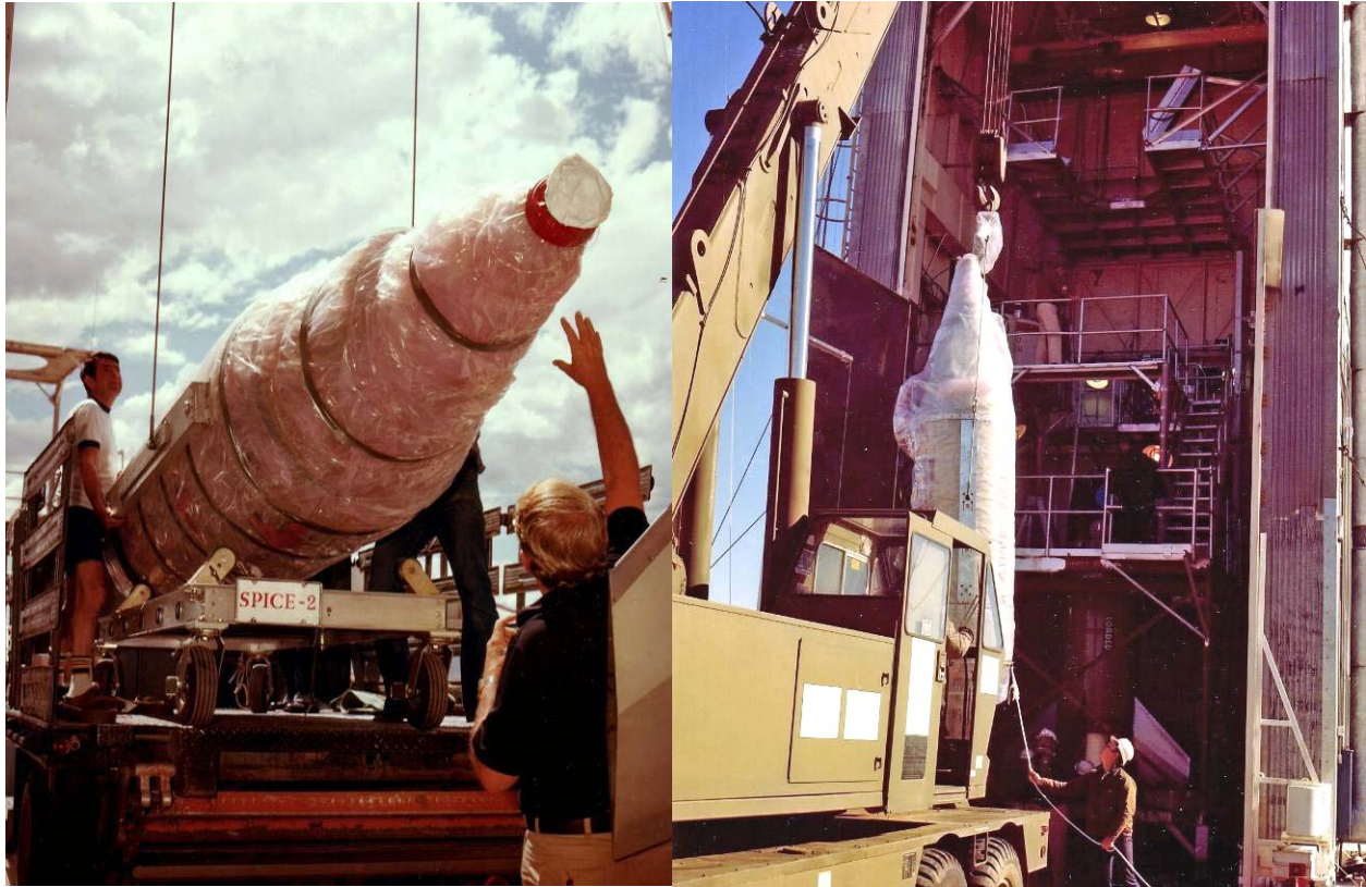
Figure 48. Payload preparations for launch. The ensuing series of images follow the sequence of launch preparations using a montage of photographs from the SPICE and FIRSSE experiments. Above left, the cleaned and bagged payload has been loaded on a cart on a pickup truck to be taken to Launch Complex 36 at the White Sands Missile Range. It is shown here as it is being lifted off the truck. The right hand picture shows the payload being hoisted into the roll away launch preparation building.
