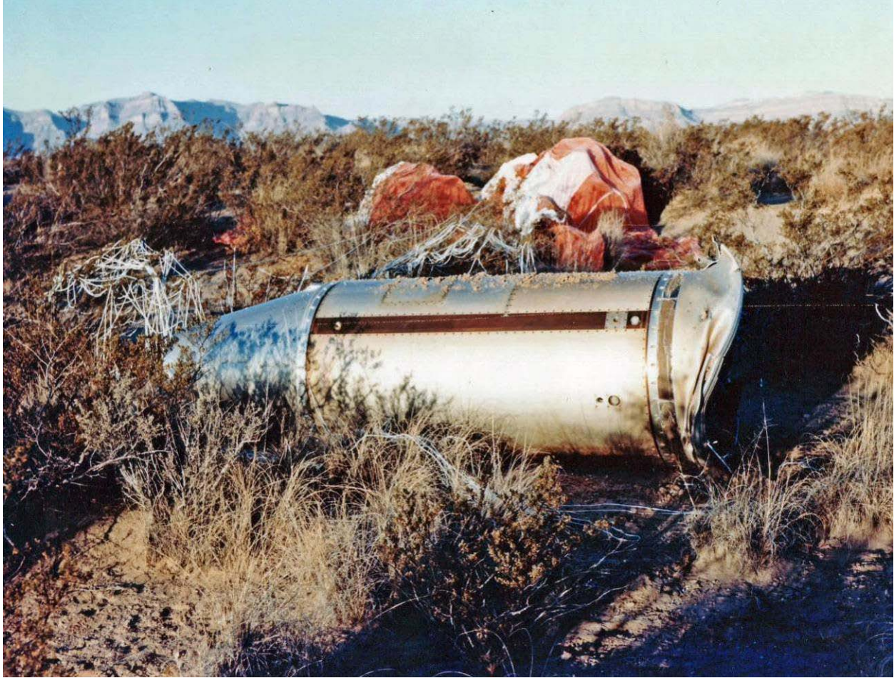
Figure 43. The not so soft SPICE I recovery. The payload impact was much harder than anticipated with the standard recovery pack used on this mission. Despite the appearance, the internal damage was limited.
