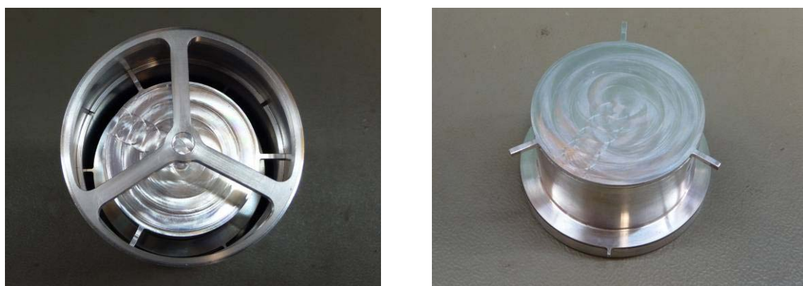
Figure 15: Top hat with reduced diameter and machined locating tabs
