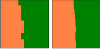
Figure 3: Comparison of two algorithms to interpolate the labels, after two consecutive interpolations. Left: interpolation followed by thresholding. Right: our proposed simple approach.
