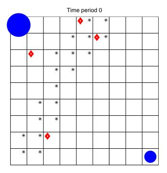
Figure 1: Area of interest with diamonds indicating initial location for moving targets, asterisks indicating difficult-to-search cells, and circles indicating initial locations of searchers. The number of searchers is proportional to the radius of a circle.
