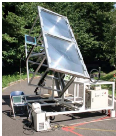
Fig. 19 – Example of simple demonstrations of direct solar pumped lasers [71]
