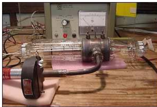
Fig. 15 – A 2 kW 5.8 GHz klystron tube developed by Ebeam for NASA
