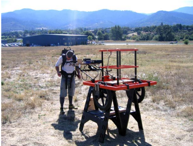
Figure A- 1. EM63 cart on sawhorses for static background test at the Ashland Test Plot.
