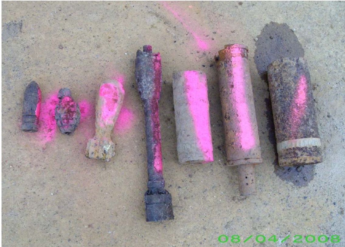
Figure 10. Photograph of the seven items measured in the test-pit. From left to right: 37mm projectile, hand grenade, 60mm mortar, 2.5” rocket, 75mm shrapnel round, 3” stokes mortar and 3.8” shrapnel round.
