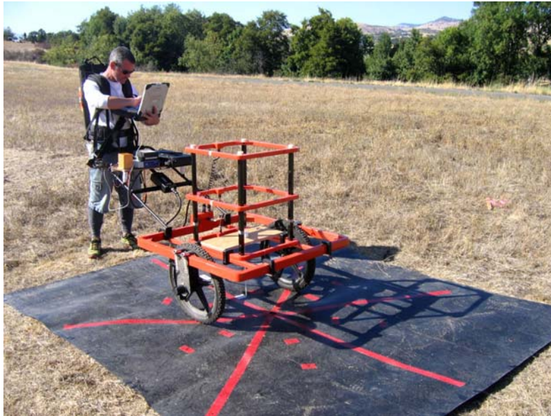
Figure 1(a) Standard EM63 cart collecting discrimination mode data at the Ashland test-site. A rigid fiberglass indicator rod is mounted in the center of the coil to accurately log the survey location. Along with the inclusion of the IMU for orientation, this minimizes positional errors.
