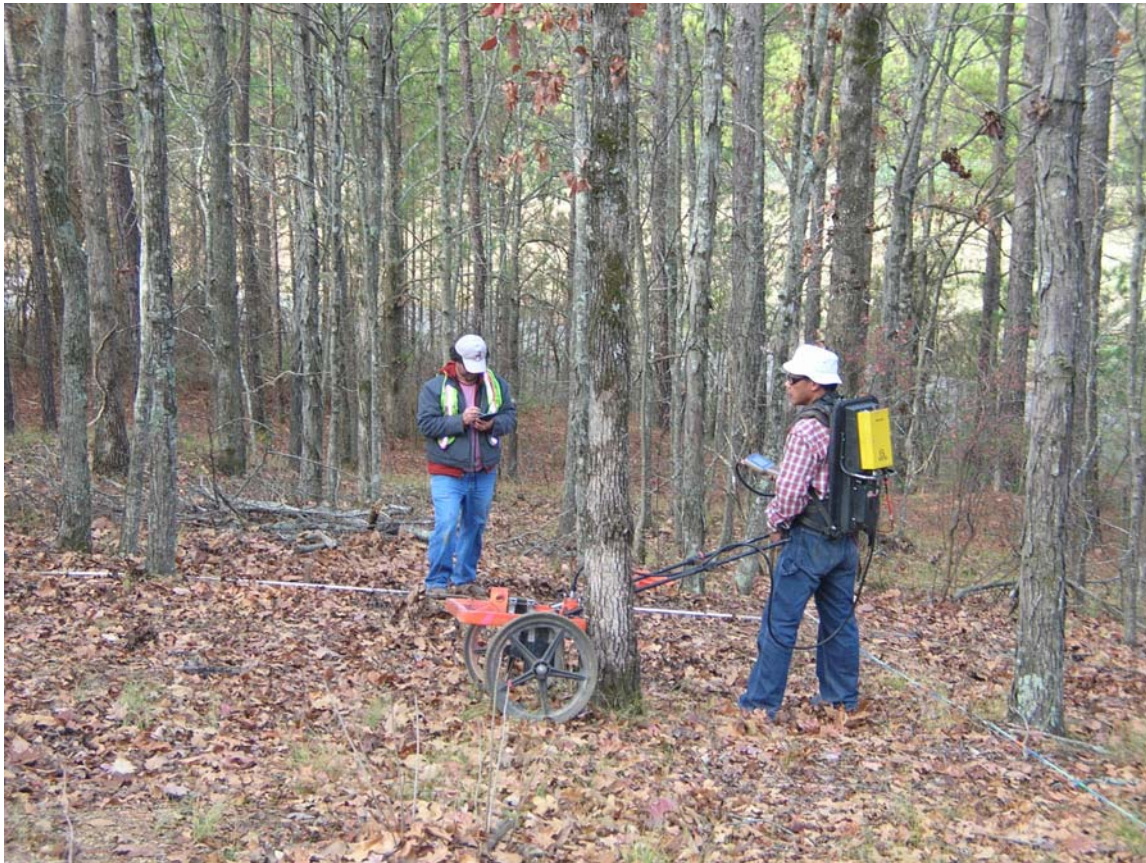
Figure 9. NAEVA crew collecting EM61 data at Fort McClellan.
