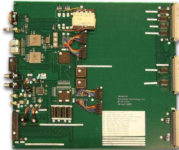
**Figure 2a - DRFM/FIR Filter Board**
