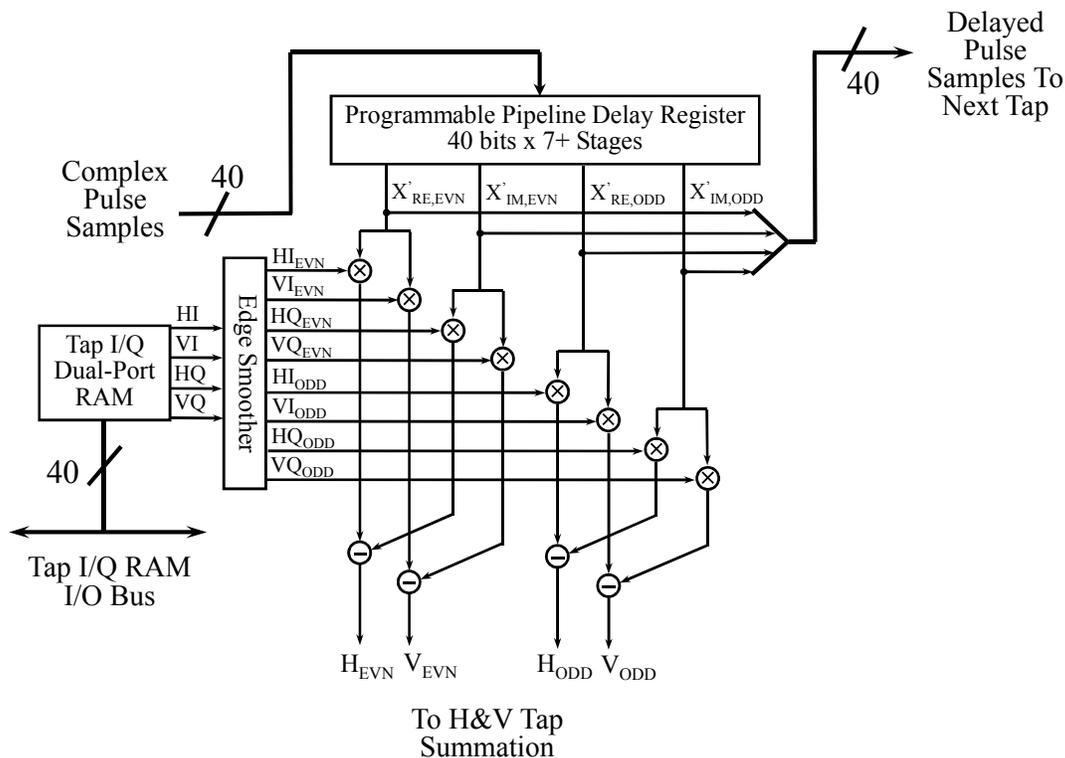
**Figure 5 - Details of Digital Tap Cell**
