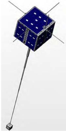
**Figure 47 - NittanySat with gravity-gradient boom deployed.**
