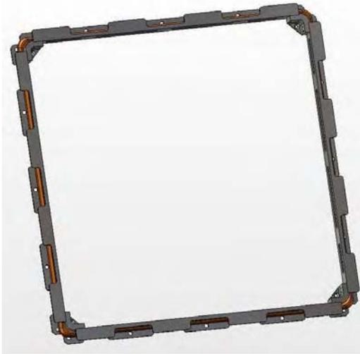
Figure 45 - Single magnetic torque coil.
