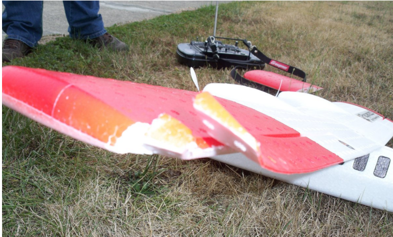
Figure 1.15: Damage on the left wing due to a mid-air collision during test flights.
