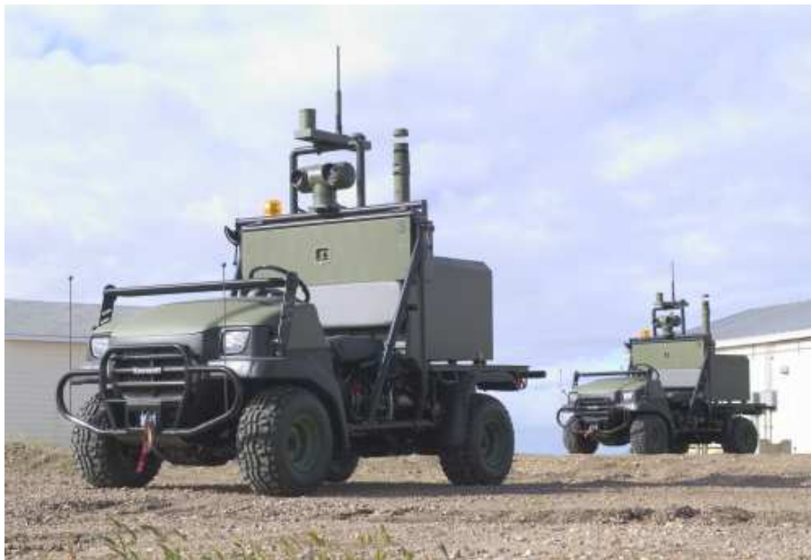
Figure 3: The Multi-Agent Tactical Sentry (MATS) robotic vehicle.
