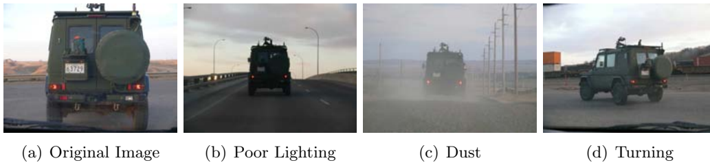
Figure 2: Some of the difficulties for an autonomous convoying vision system.
