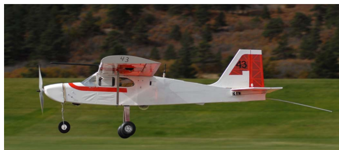
Fig. 1. Autonomous UAV platform outfitted with RF and camera sensors.
