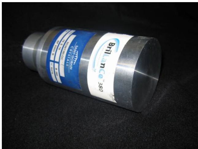
Figure 2.3-2. The 3-inch by 3-inch LaBr 3 detector received from Saint-Gobain (France).
