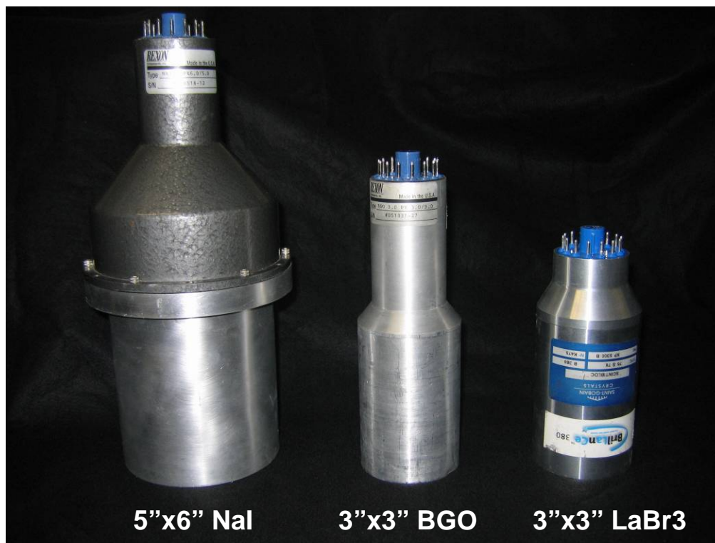
Figure 2.5-2. The three detectors used in the lab testing.
