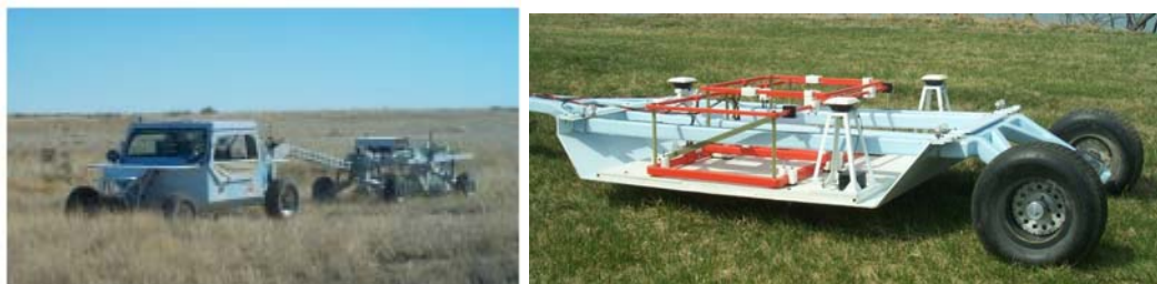
Figure 4. Naval Research Laboratories Multisensor Towed Array Detection System (left: magnetomer array, right: EM61 MK2 array).
