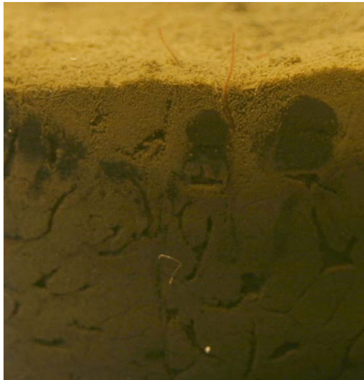
Figure 8. A close-up image of the sediment profile showing the buildup of worm feces (in 7 days) on top of the amendment pellets and the slow incorporation of the pellet materials through the worm burrows.
