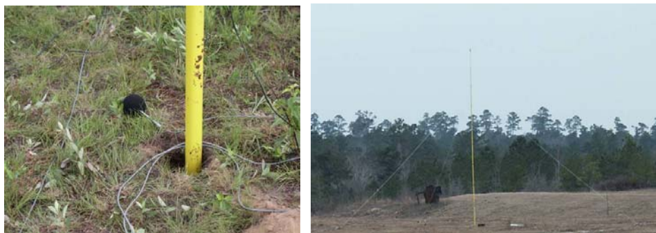
Figure 2-2. Photographs of Microphone Placement in the Field: Ground-based (left) and Pole-Mounted (right)
