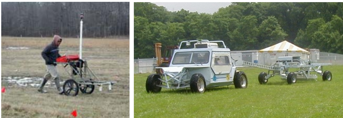
Figure 7. Shaw pushcart magnetometer system (left) and MTADS towed magnetometer array (right).
