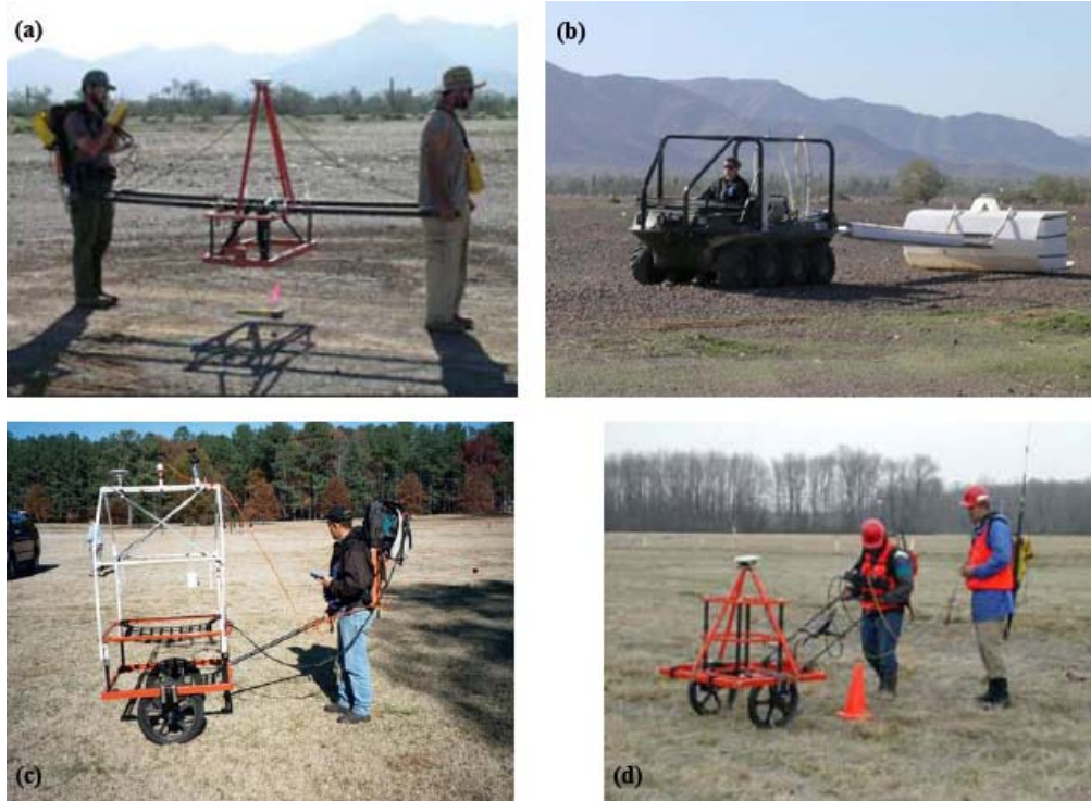
Figure 3. EMI demonstration systems: (a) NAEVA Geophysics manportable EM61, (b) NAEVA Geophysics EM61 towed array, (c) TtFW EM61, (d) ERDC EM63.
