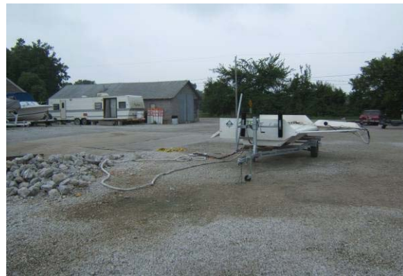
Figure 6-6. The sensor platform is assembled on its boat trailer, the tow cable is coiled up on top of the platform and it is launched beside the pontoon boat for mating.
