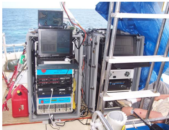
Figure 7-7. The MTA electronics racks are shown mounted on the Coral Queen. The ladder in the foreground leads up to the flying bridge.
