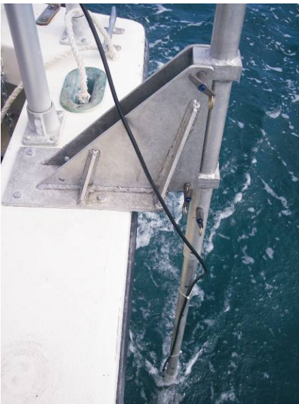
Figure 7-8. On the left the mount for the sonar altimeter is shown attached to the port rail. On the right the pilot guidance display is shown mounted on the bridge in front of the driver.
