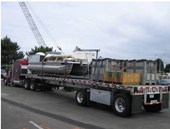
Figure 5-7. All of the MTA system components were shipped on the deck of a single 45 ft trailer. The sensor platform was transported on the boat deck.
