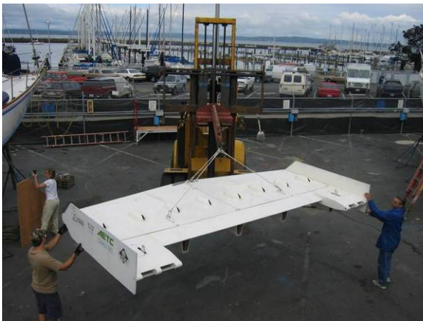
Figure 5-9. A large forklift was used to unload the sensor platform and later load it back onto the MTA vessel boat trailer.
