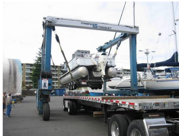
Figure 5-8. A marine hoist was used to unload the MTA vessel and the trailer together. It is difficult to lift the vessel alone without damaging the pontoons.
