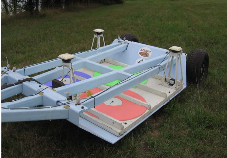
Figure 2-4 MTADS GEM array mounted on the EM sensor cart. In addition to the three GEM sensors (false colors to identify coils), note the three GPS antennae and the inertial measurement unit (under GPS receiver near back left tire) for platform motion measurement.
