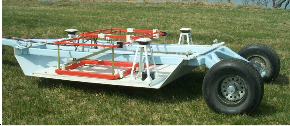
Figure 2-3 Close-up of MTADS EM61 array with GPS and IMU
