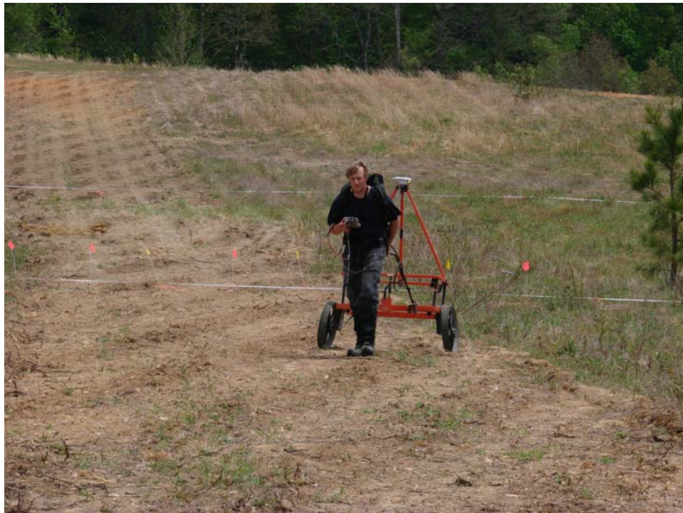
Figure 4-1 Photograph of the EM61 MK2 Cart
