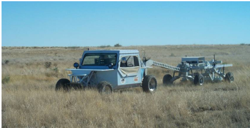
Figure 2-1 MTADS tow vehicle and magnetometer array
