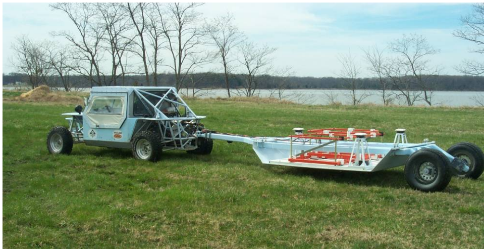
Figure 2-2 MTADS EM61 array pulled by the MTADS tow vehicle
