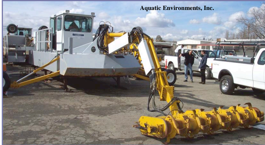
Figure 5-4. AEI “Aquamog” with rotovator arm
