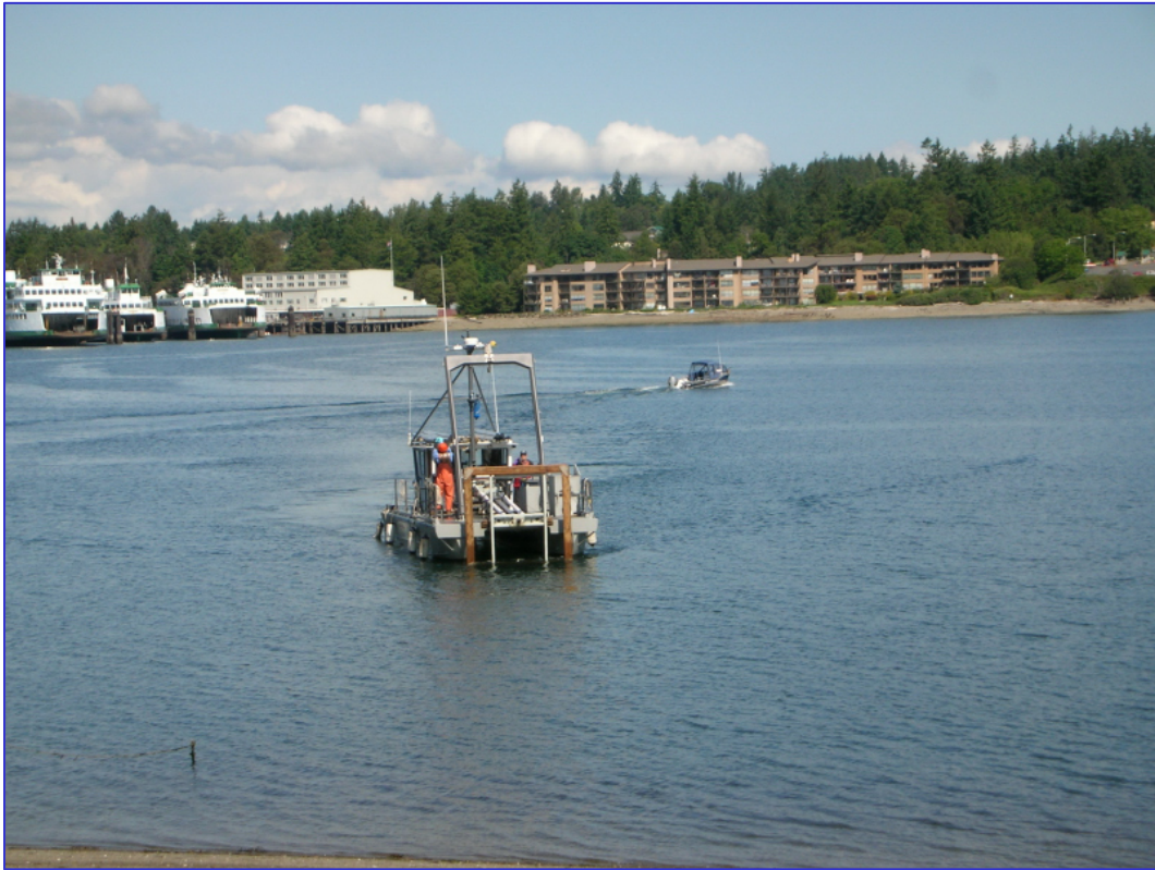
Figure 3-4. Vibracoring Activity on the Cap at Eagle Harbor
