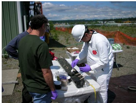
Figure 3-8. Porewater Sampling and Core Segmentation Processes in the On-Site Processing Area
