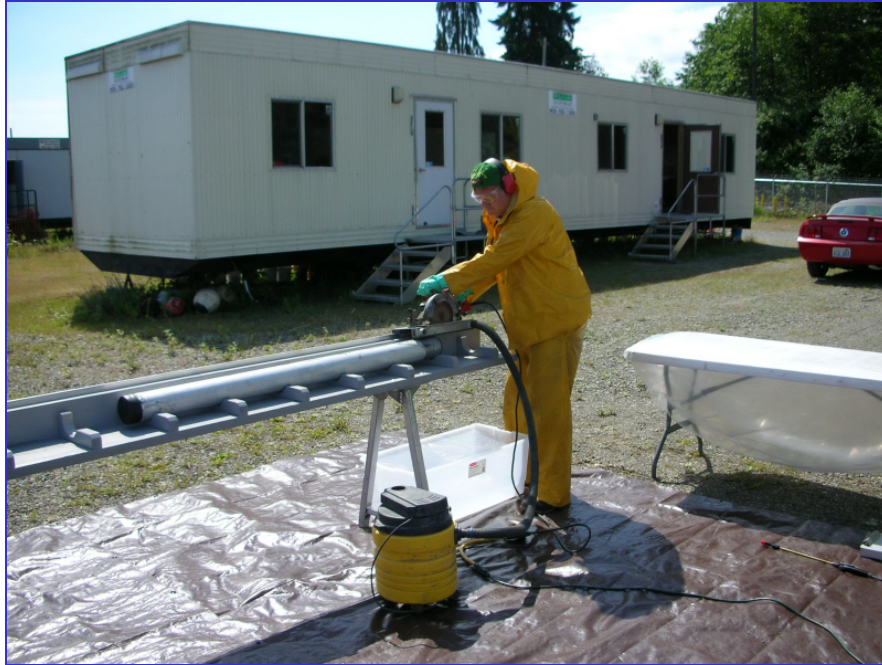
Figure 3-6. Opening the Aluminum Core Tube for Sediment Core Processing Using a Circular Saw
