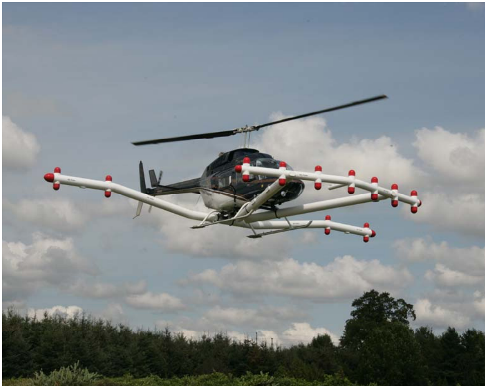
Figure 2-3. VG-22 airborne vertical magnetic gradient system.
