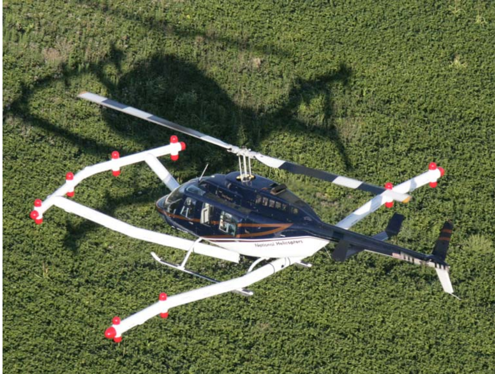
Figure 2-2. Battelle's VG-16 airborne vertical magnetic gradient system.
