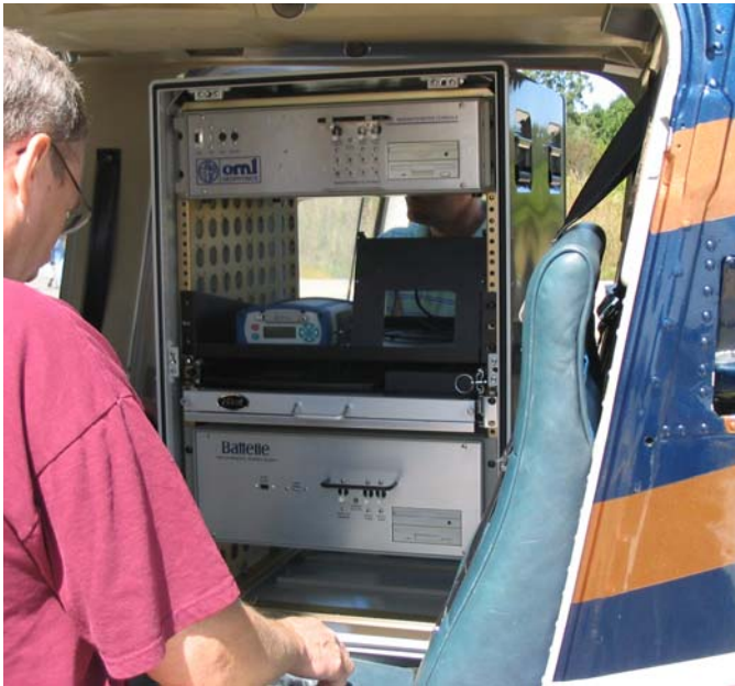
Figure 2-1. Recording equipment rack-mounted in the helicopter for both systems.
