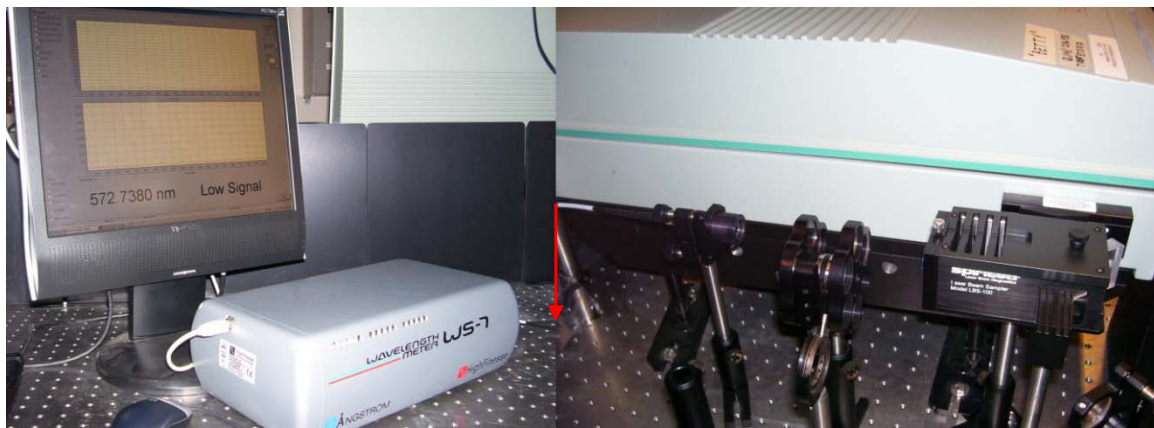
Figure 18. Checking wavelength using wavemeter
