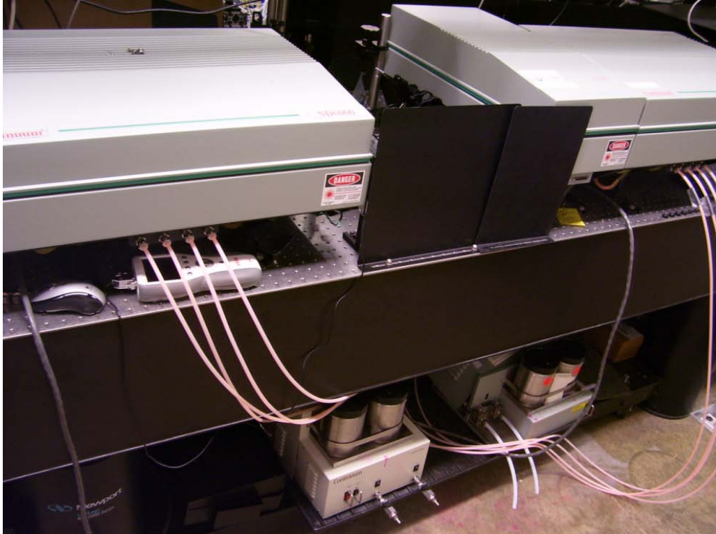
Figure 17. ND6000 narrowband dye laser with frequency doublers
