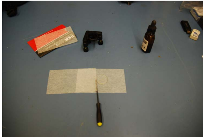
Figure C-3. Drop and drag cleaning method
