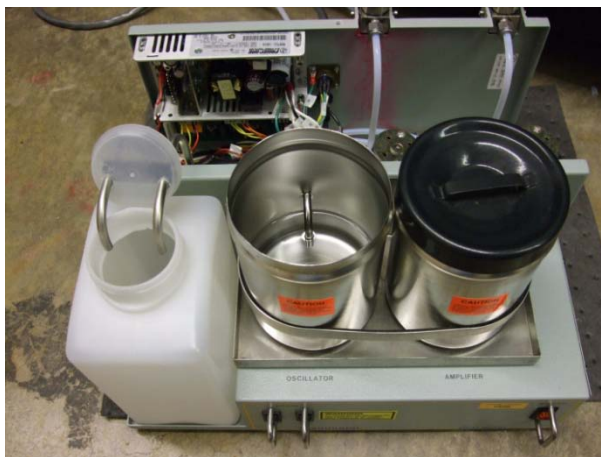
Figure A-3. Dye pump for dye laser
