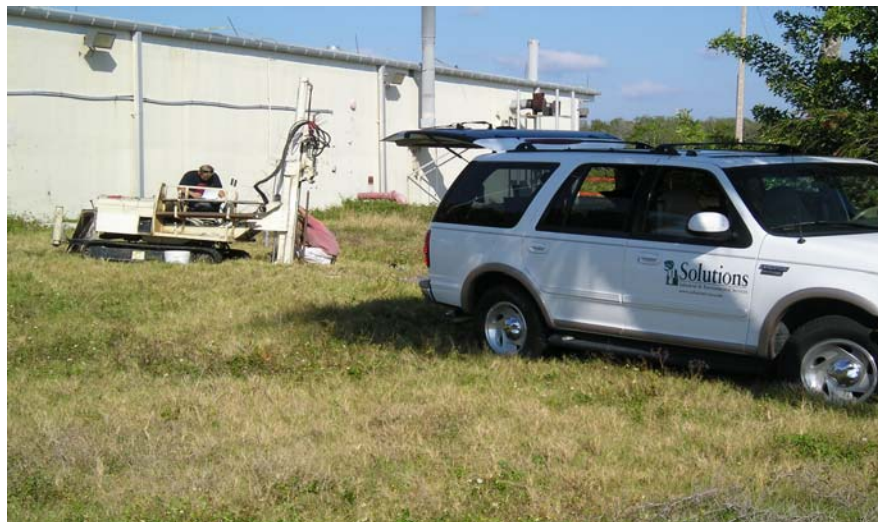
Figure 6-4. Sample Collection using Geoprobe beside the Engineering Support Building
