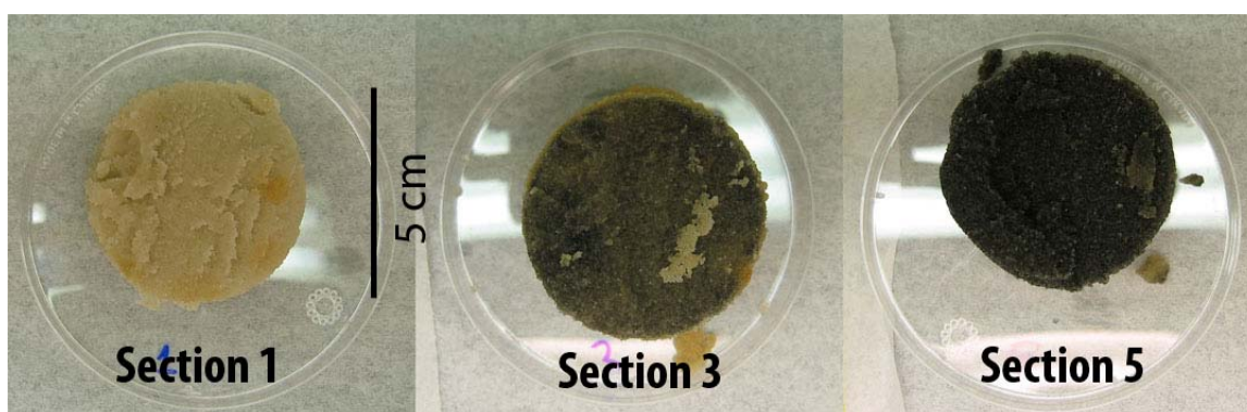
Figure 4.20. Sections taken from the FeS-coarse column indicate dissolution of FeS, but no preferential flow paths. Each section is 2.5 cm thick, and section 1 is the influent end of the column.
