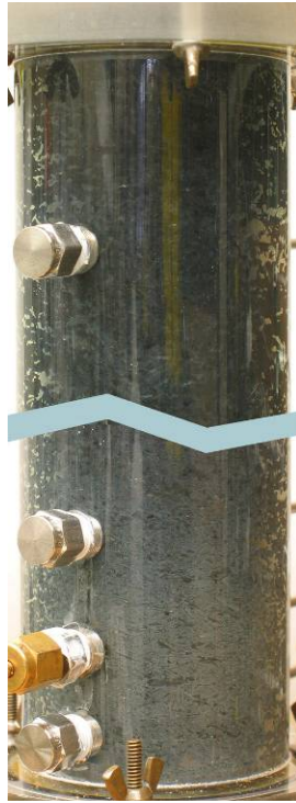
Figure 4.17. Change in color in the ZVI column influent end (bottom) relative to effluent end suggests accumulation of calcium carbonate.
