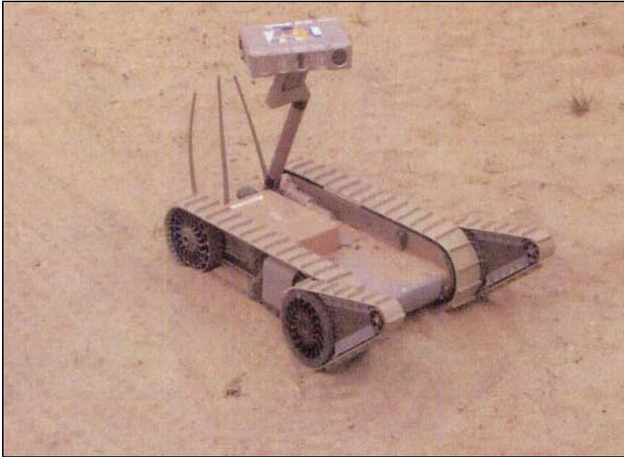
Figure 7. The iRobot PACKBOT Explorer.
