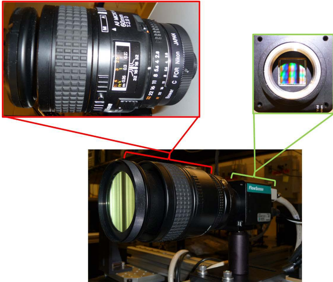
Figure 8. Flowsense 4M camera showing filter, lens, and CCD
