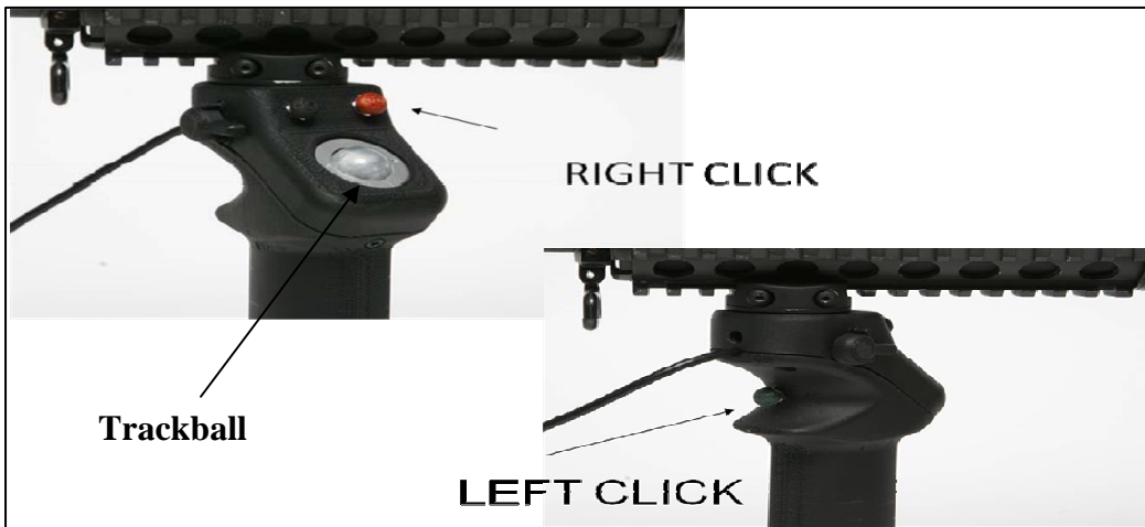
Figure 2. System A control locations.
